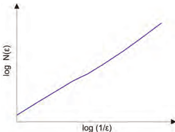
Text-fig. 8. Fractal dimension. If we plot \log(1/\epsilon) against \log N(\epsilon) , the fractal dimension is given by the gradient of the best fit line
